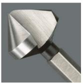
1-flute countersink bits, 90° • Application: Deburring, chamfering and countersinking • ¼" drive suitable for holders as per DIN 3126-D 6.3 (ISO 1173) • Hexagon shaft for very high torque transfer • 1 tip • Guaranteed vibration-free and scratch-free operation • Optimal countersink surface quality • Long service life • Perfect chip removal • High corrosion protection
