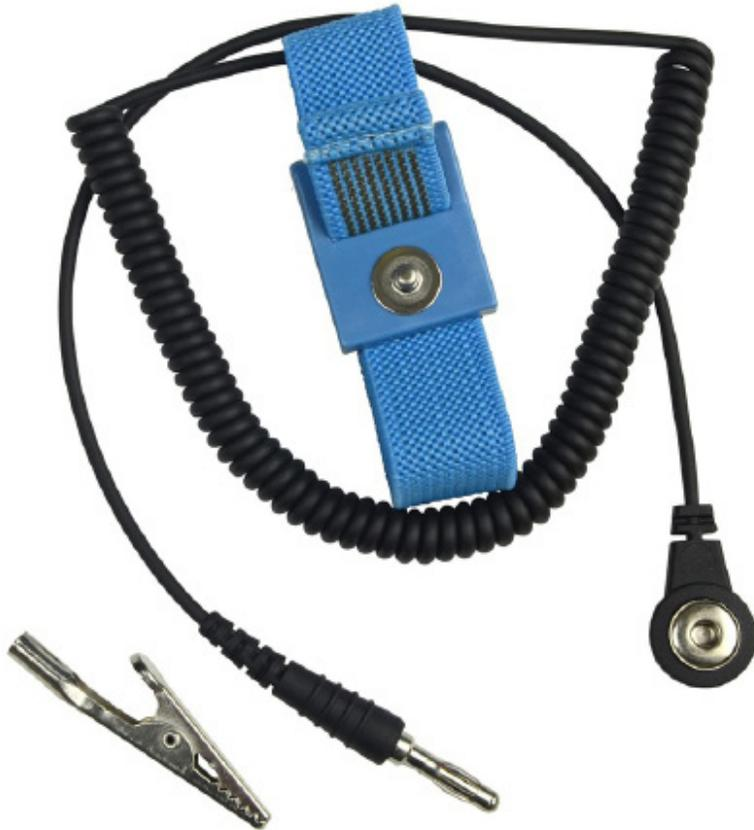
This SCS Economy Single-Wire Adjustable Wrist Strap set provides a cost-effective means of grounding production employees. This wrist strap features an adjustable fabric wristband with a 6-foot retractable coil cord, alligator clip and a 4mm snap. Meets ANSI/ESD S20.20 and ANSI/ESD S1.1.
