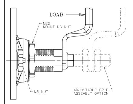
COMPRESSIVE STRENGTH - MAXIMUM WORKING LOAD: 445 N (100 lbf) \* - AVERAGE ULTIMATE LOAD: 1112 N (250 lbf) \*
