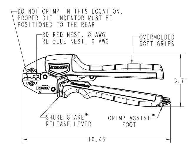
CAUTION: HANDLES NON-INSULATING, DO NOT CRIMP ENERGIZED WIRES
