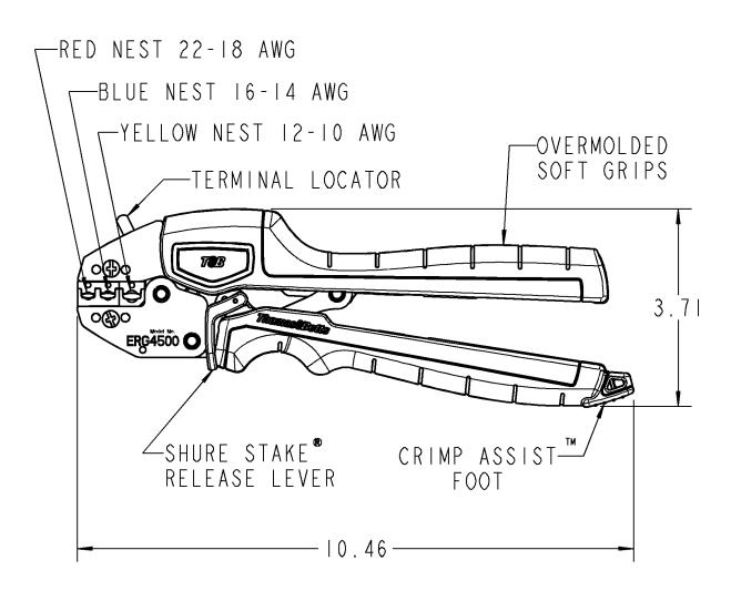
CAUTION: HANDLES NON-INSULATING, DO NOT CRIMP ENERGIZED WIRES
