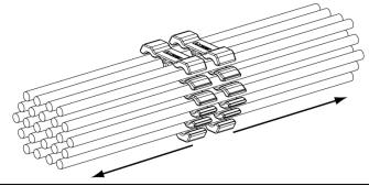
STEP 4: After the inserts are separated, install the hinged jacket around each insert and secure with the attached hook and loop fastener to secure the assembly. Each of the tools can now be guided in either direction to organize cables. Apply cable ties at desired intervals as you move along the cable bundle length.
