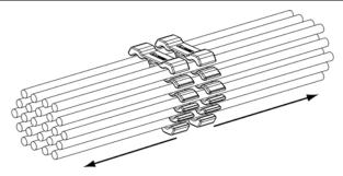
STEP 4: After the inserts are separated, install the hinged jacket around each insert and secure with the attached hook and loop fastener to secure the assembly. Each of the tools can now be guided in either direction to organize cables. Apply cable ties at desired intervals as you move along the cable bundle length.
