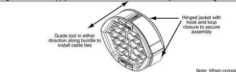
Note: When complete slide reusable tool off of cable bundle
